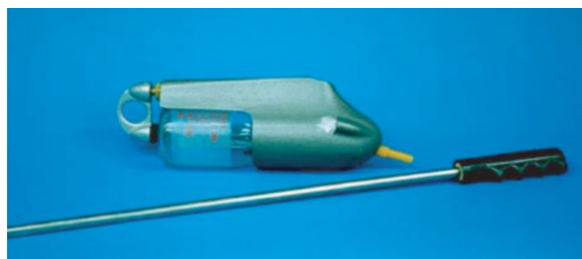
Fig. 2. US-DH 48 sampler used for suspended load data collection
